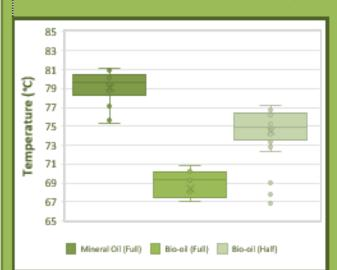
As these results show, bio-oil (even at a lower flow rate), clearly operates at cooler temperatures compared to normal mineral oil
