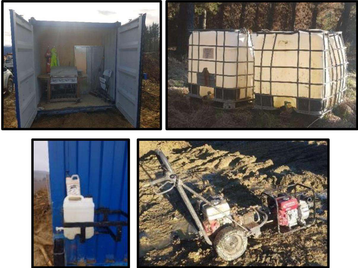
*Figure 1. Reed Contracting (clockwise from top left): a) the storage at the end of the hut houses wet weather gear, other PPE, clean drinking water, a BBQ and a heater (when not in use); b & c) water tank, blaster and pump are used for washing down all machinery before it's transported between sites, or in some cases between waterways to prevent the spread of Didymo; and d) soap and water by the entrance to the container so that the crew can clean their hands.*
